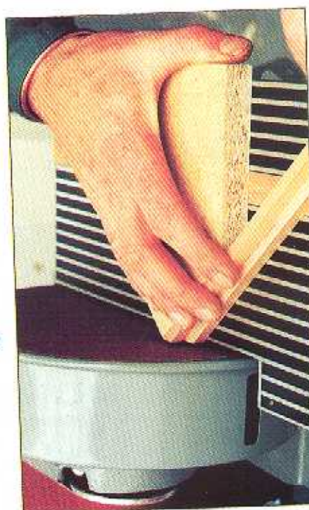
Trimming the sawn mitre cut using a mitre shooting board. Note the wafer-thin end grain shavings produced by the sharp plane blade.
