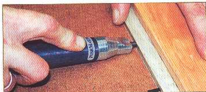
The backing board is held in place using flat plates or small panel pins.
