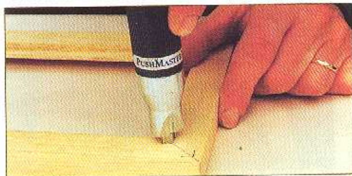
Reinforcing the mitre joints using the nails inserted with the Push Master.
