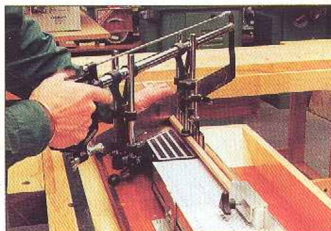
Cutting the mitres using a mitre frame saw.
