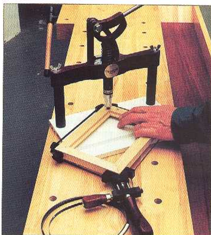
A strap clamp in operation while the nails are inserted using the Push Master mounted in a cam-operated jig (useful for hard timbers).
