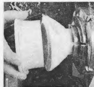
4 Turn the lip to the scribed line. Check the fit as you work. The lid should fit loosely because the wood will shrink and expand.
