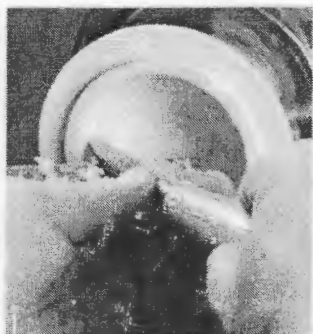
6 Cut a step for the chuck jaws. Similar to the base, cut an angled step on the inside of the lip for the expanding chuck jaws to grab before removing the lid and remounting it. Apply a finish to the inside surface.
