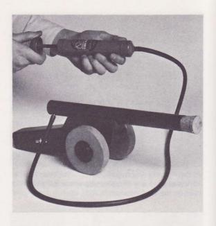
Make the gun carriage according to the pattern below. Round out the V-groove in it with sandpaper wrapped around the barrel and bed the barrel with epoxy cement. Glue on the wheel spacer blocks.
