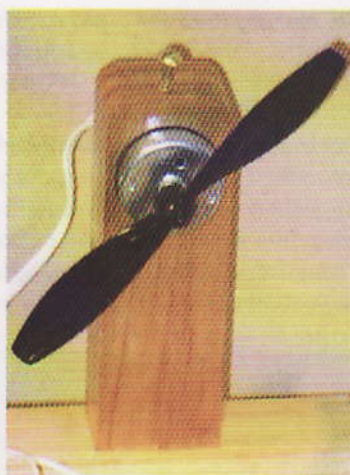
The motor mounting will have to be constructed bearing in mind the specific motor and propeller that you obtain.
