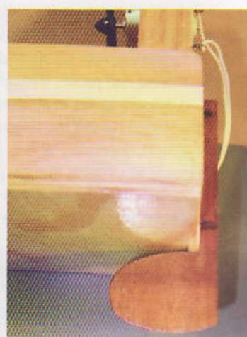
The fixed rudder is made from hardwood and glued to a plywood plate which is attached to the stern with small brass screws.
