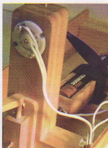
The motor may not be marked with which terminal is positive, so determine this by trial and error.
