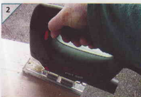
2 You can use a standard blade for a curve such as this, but when cutting sharp curves use a narrower blade.
