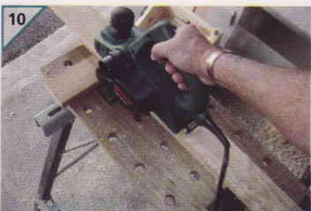
Plane the drawbar slightly to allow it to slip easily between the underside of the seat and the rear axle assembly.
