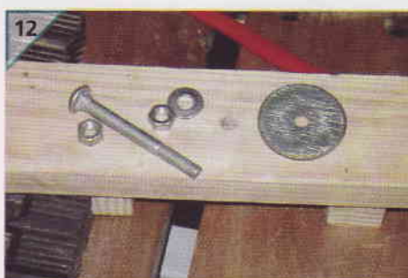
Use a large flat washer between the front axle strut and drawbar, so that you have a large bearing surface.
