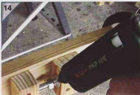
Use locknuts (two nuts tightened against each other) and a proprietary product or hot glue to lock the nut in position.
