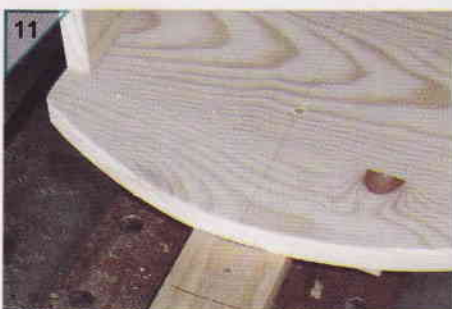
The two holes (at 150mm centre to centre) in the seat guide you in drilling the holes in the drawbar.
