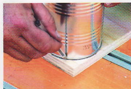
Round off the corners on the front side of the seat.
