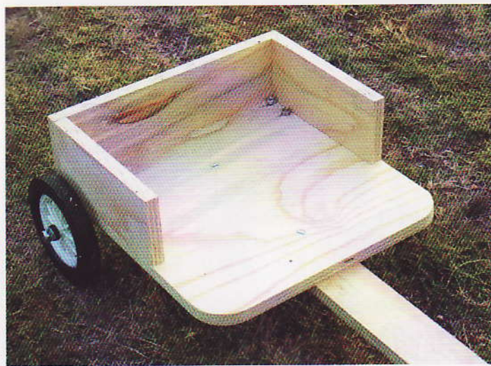
❶ The seat was assembled with dowels, that in the event of an accident, would be safer than exposed screws.
