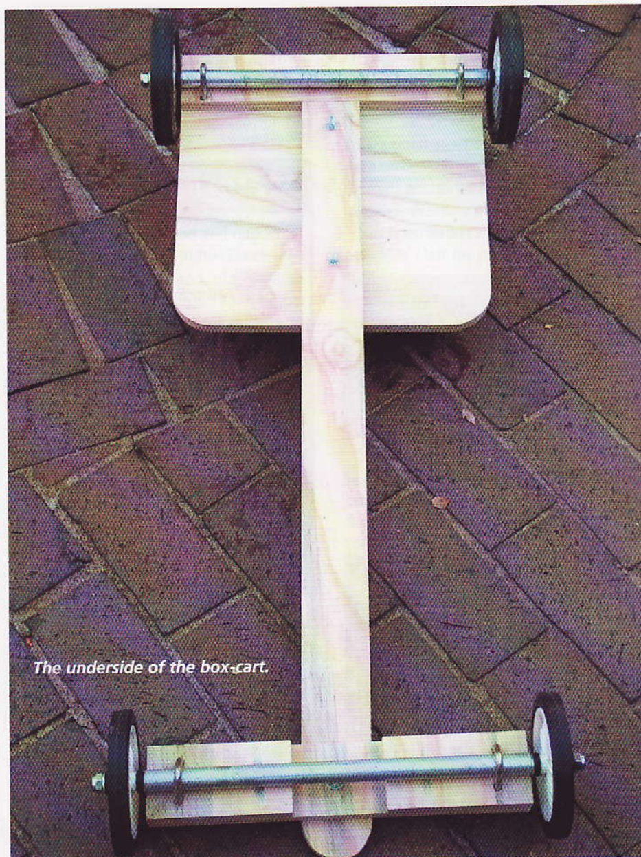
Ellis U-bolts holding the galvanized pipe in position.
