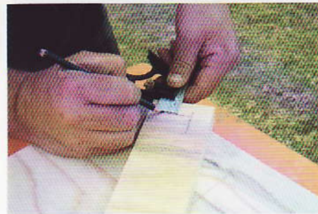
Mark out the thickness on the back and side pieces on the spacer to enable you to drill the holes as close as possible to the sides of the seat.
