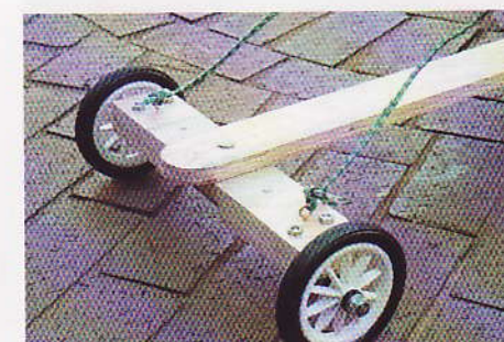
The completed steering mechanism.
