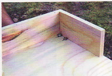
This is the desired position for the U-bolts.
