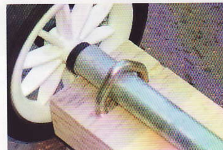
Ellis U-bolts holding the galvanized pipe in position.
