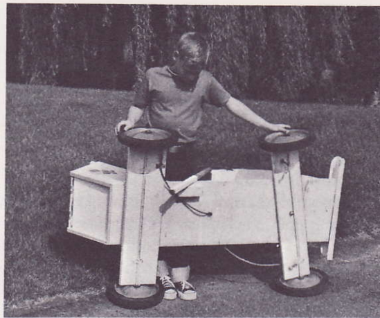
Chassis view shows how speedometer cables goes out bottom and back to rear wheel. Rear axle board is nailed to chassis, front one bolts to plywood
