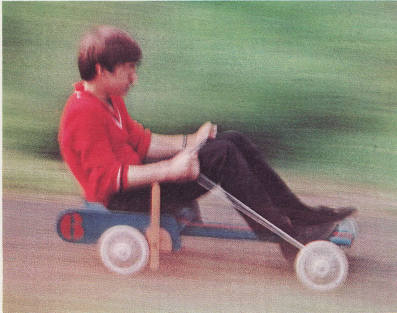
The trolley can be steered with the feet while the hands apply the brakes.
