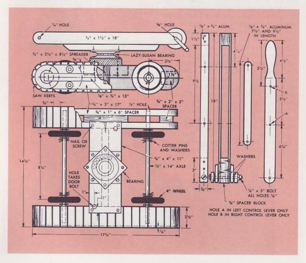
between the winch drum and the boom mount so the drum can move endwise permitting a bolt at the end of the crank to slide between two pins on the boom mount to lock the winch. Nylon cord is fastened to the drum and is provided with an S-hook made of No. 11-ga. wire, for easy attachment to objects to be pulled. When not in use the cord is wound up on the drum and the S-hook is clipped in a screw eye on the cab.
