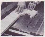
A 7° BEVEL is cut along both edges (left). Note that, after you have cut one side, board must be flopped before cutting second edge to insure that bevel angle is properly positioned. 35° bevel on top of cradle sides is cut (right) after pieces have been separated.
