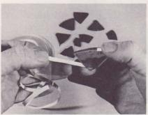
CAREFULLY center copper foil on edges of each piece of glass and wrap it tightly. Then smooth foil with dowel. Foil won't stick to greasy glass.
