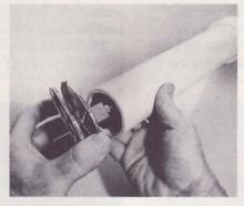
**CEMENT** end cap and acrylic eyepiece to one end of tube, and cement the glass assembly into the other end. Clean parts before assembly.
