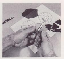
**SNAP GLASS** immediately after scoring it, using a downward and outward motion. Use pliers to break off small pieces. Rub edges of two pieces together to dull any sharp spots.
