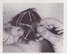
ASSEMBLE revolving unit; it consists of two glass wheels, acrylic disc, a wood block, bolt and nut.
