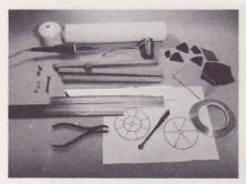
MATERIALS from top: 2-in. inside diameter plastic pipe and end cap, soldering iron, 50/50 solder, stained-glass scraps, copper spacers, bolt, washers, wood strips, wood block, mirror strips, acrylic circles, glazier pliers, pattern for stained-glass wheels, glass cutter and copper foil.
