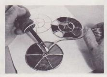
AFTER POSITIONING glass pieces on pattern and fluxing copper foil, run a bead of solder along edges, using a 60-to 100-watt iron. Then solder a piece of copper tubing in center as a spacer.
