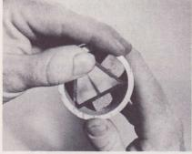
SLIDE MIRRORS into tube so they form a triangle, mirror side facing inward. Wood strips that hold mirrors should fit snugly, but be careful not to scrape any of the backing off the mirrors.
