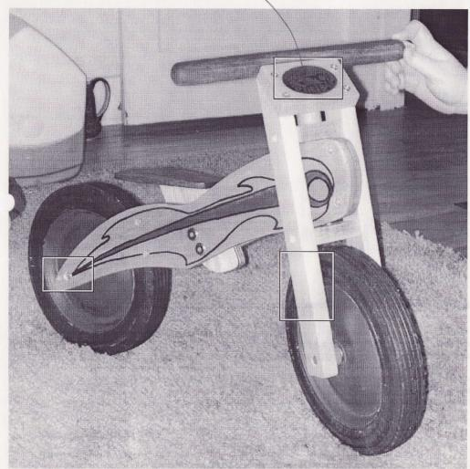
Fortunately, my office has a printer with a straight-pass feeder designed for CDROM's. So, I printed the logo onto a copper disk that I hand cut into the size of a CD. Then, I coated the disk with polyurethane, cut it into an oval badge, and epoxyed it on the front of the bike. (You can also see how I re-designed the front forks to accommodate the ½" axels.)
