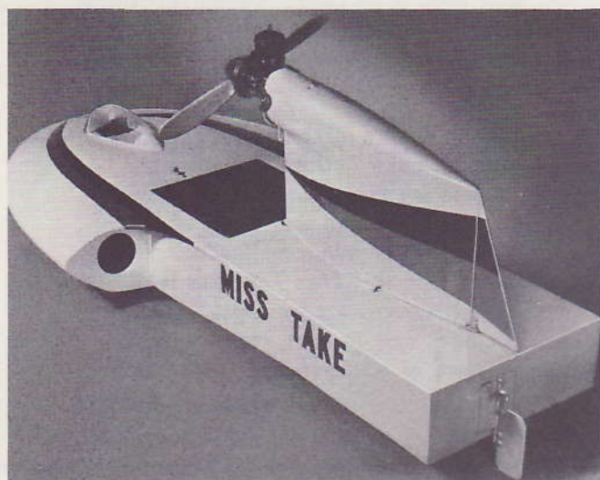
The double rudder system is shown in this view of Miss Take . The air rudder serves as a low-speed backup to the water rudder, is effective at high speed
