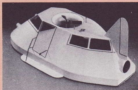
Top and rear views above and below show the engine mounted in the intake duct and the propulsion tube outlet at the rear. Note the wire hook on the door for tethering
