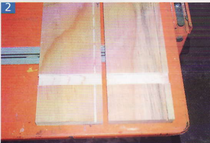
The wood cleared from between the two cut lines to make the joint – a depth of about 6mm will be sufficient.
