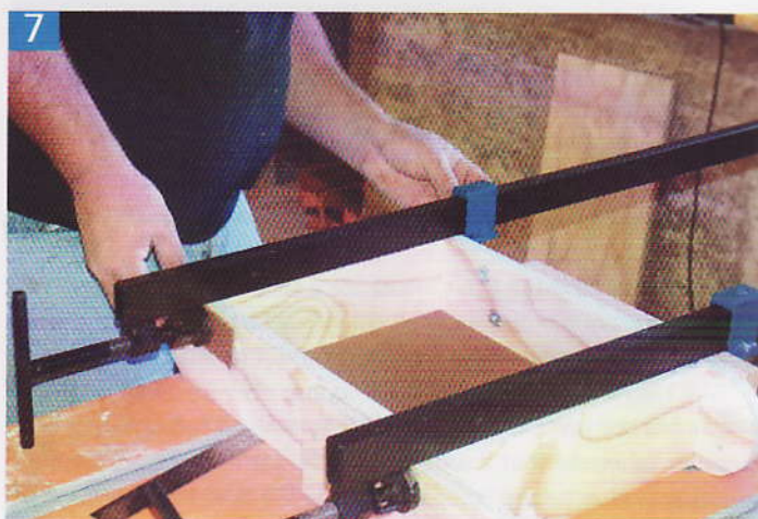
Use sash clamps to clamp the box while the glue dries.
