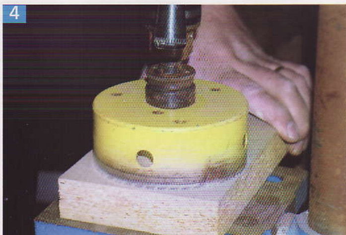
The wheels being cut with the hole saw.
