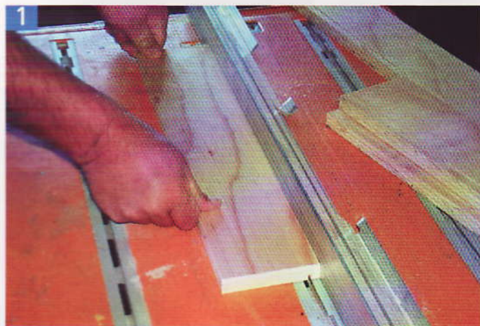
The groove being cut about 6mm deep into the sides for the base to slide into. Relace the rip fence once finished.
