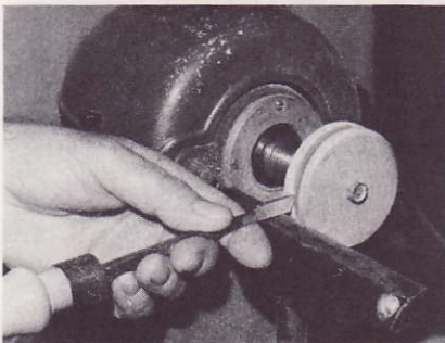
CABLE GROOVE in sheave is turned so it will accommodate two turns of cable.
