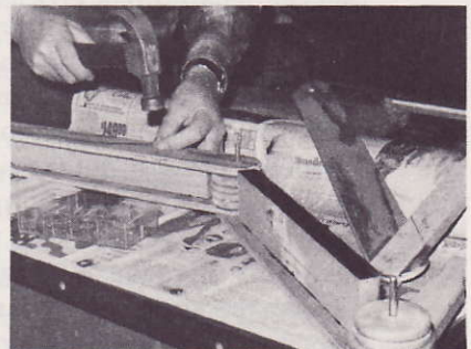
BOOM AND ARM are assembled with axles and sheaves in place temporarily.
