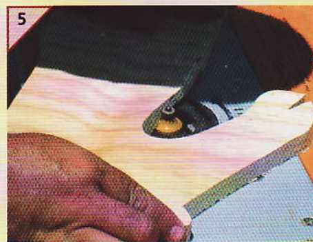
Rout a round edge onto the head making sure you do not rout too far down the neck as this will look odd once the sides are connected.
