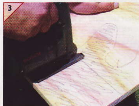
3 Cut out the head using a jigsaw.
