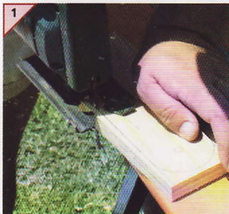
1 Start the project by cutting all your timber to size – here the legs are being cut.
