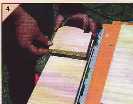
Gluing the sides for the horse body.
