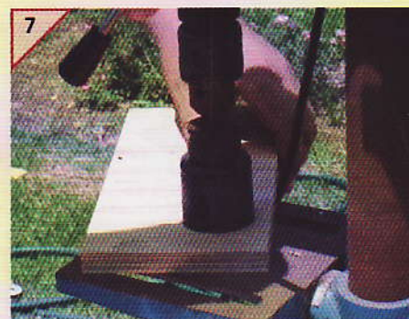
Drill the holes for the eyes, handle and the locating dowels that position the legs and shoulder discs using the hole saw.
