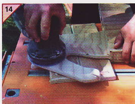
14 Sand all the pieces of the horse before the final assembly.
