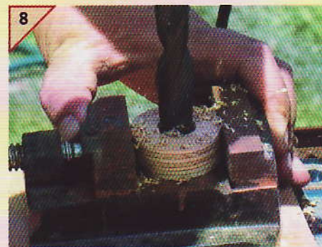
Use the hole saw again to cut four discs and then drill a 19mm hole through the centre of each.
