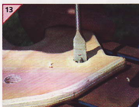
13 Drilling the eye hole for the horse.
