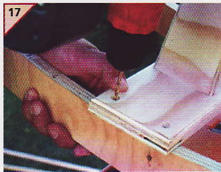
17 Attaching the rocker brace to the rockers.
