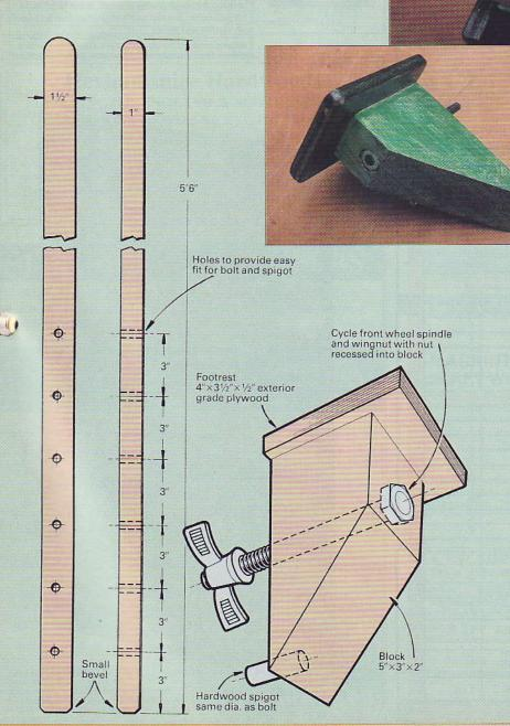
The height of the footrests on the poles is adjustable as there is a series of holes for locating these using bolts and wingnuts and spigots to prevent twisting.
