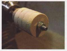
O If you do decide to make the wheels yourself, they can either be turned on the lathe or made using a holesaw. I used a combination of both. The standard pilot drill on the holesaw is 6mm, so I made a mandrel from a 6mm coach bolt.
