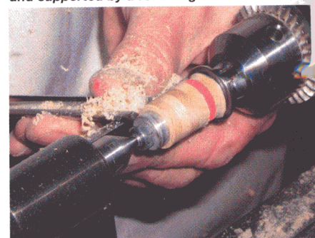
Wheels mounted on mandrel and supported by a revolving centre
