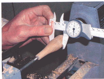
Checking the diameter with the lathe stationary
