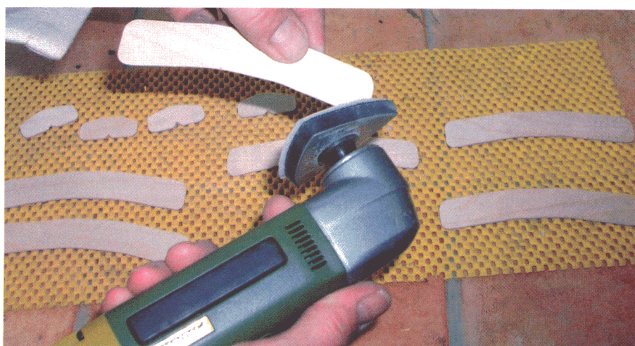
Proxxon delta sander used to remove any whiskers
