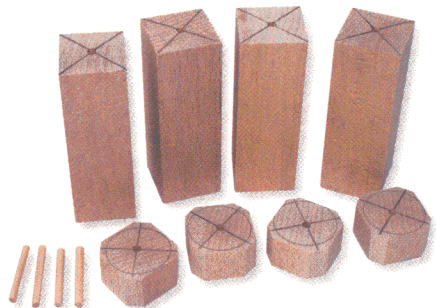
Blanks for fuselage and nose cone together with lengths of dowel
