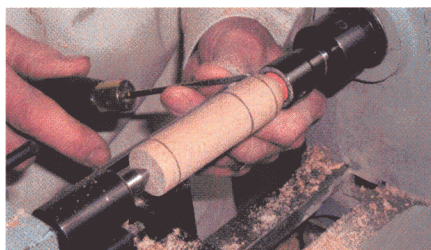
Round off front end of fuselage down to the turning guide
