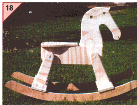
18 Almost there – all that needs to be done is the fitting of the marbles for the eyes, fitting the handle and painting.
