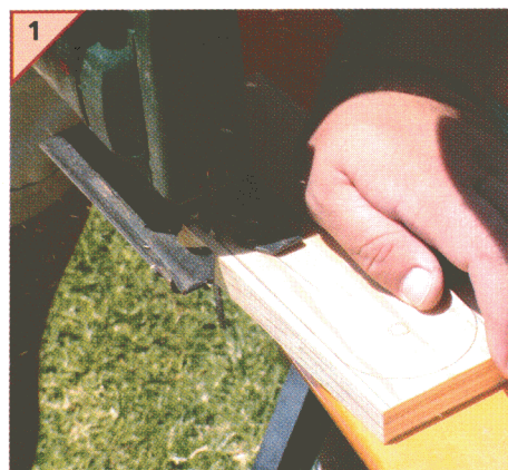
1 Start the project by cutting all your timber to size – here the legs are being cut.
