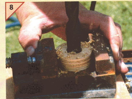
Use the hole saw again to cut four discs and then drill a 19mm hole through the centre of each.
