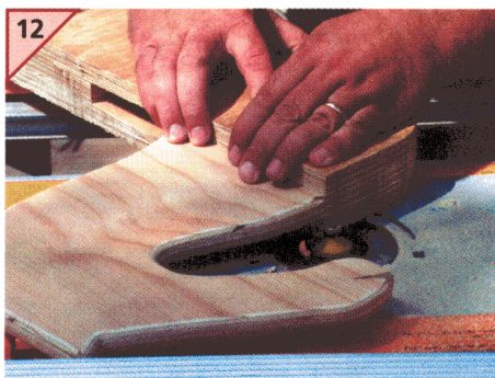
12 A rounding-over bit is used to round the sharp edge of the horses' body.
