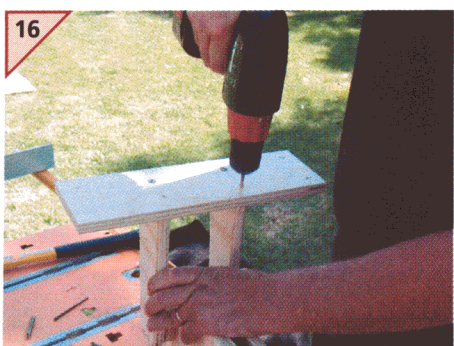
16 Fitting the back rocker brace to the legs.
