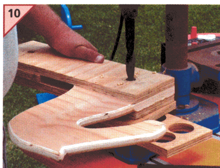
10 Using the drill press and the 19mm drill bit again, drill through the neck and sides for the dowel.
