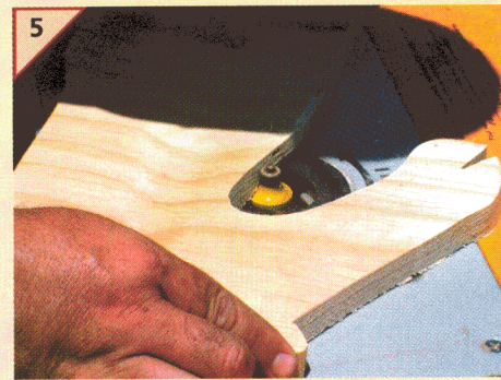
Rout a round edge onto the head making sure you do not rout too far down the neck as this will look odd once the sides are connected.
