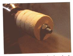
O If you do decide to make the wheels yourself, they can either be turned on the lathe or made using a holesaw. I used a combination of both. The standard pilot drill on the holesaw is 6mm, so I made a mandrel from a 6mm coach bolt.
